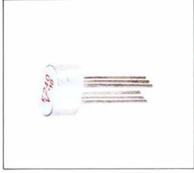
The ultralow-noise, high Gm dual FET, heart of the equalizer amp.
